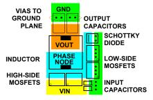
FIGURE 35. TYPICAL POWER COMPONENT PLACEMENT
