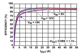
FIGURE 1. EFFICIENCY vs LOAD
