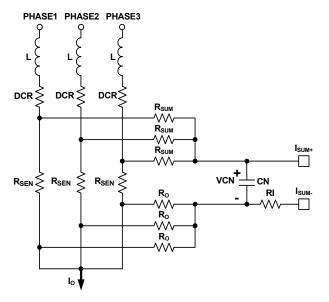
FIGURE 30. RESISTOR CURRENT-SENSING NETWORK
