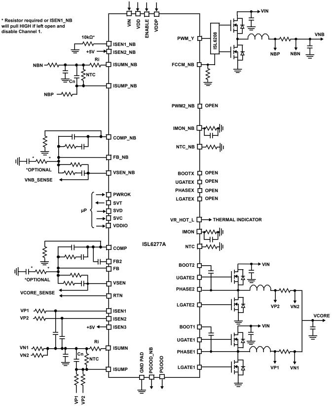
FIGURE 5. TYPICAL APPLICATION CIRCUIT USING RESISTOR SENSING
