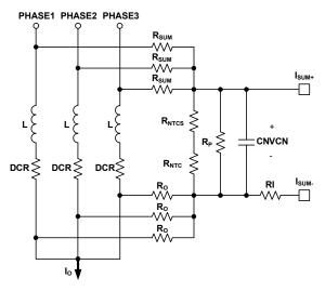
FIGURE 24. DCR CURRENT-SENSING NETWORK
