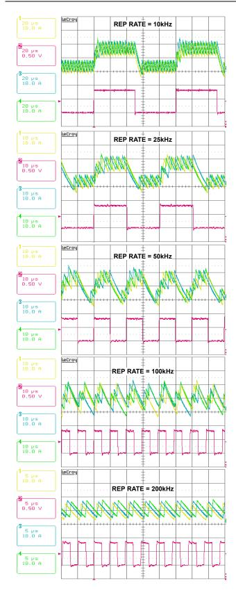
FIGURE 19. CURRENT BALANCING DURING DYNAMIC OPERATION. CH1: IL1, CH2: ILOAD, CH3: IL2, CH4: IL3
