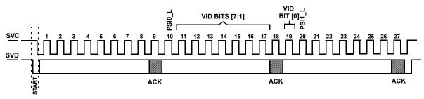
FIGURE 21. SVD PACKET STRUCTURE
