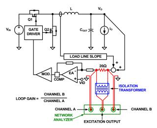
FIGURE 32. LOOP GAIN T1(s) MEASUREMENT SETUP
