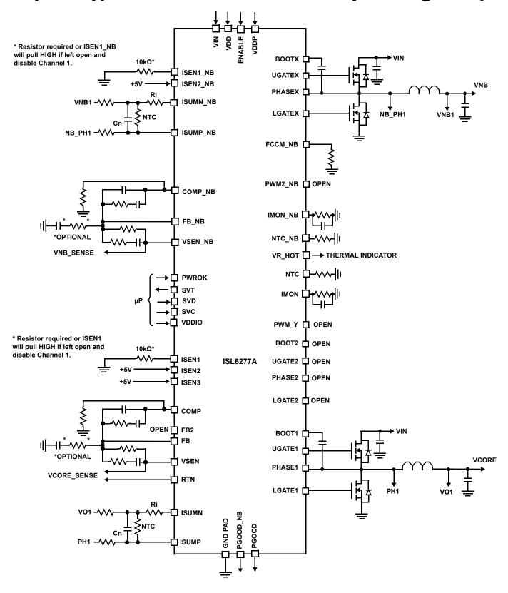
FIGURE 6. TYPICAL APPLICATION CIRCUIT USING INDUCTOR DCR SENSING
