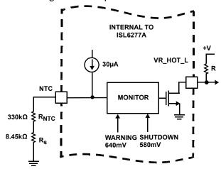
FIGURE 34. THERMAL MONITOR FEATURE OF THE ISL6277A
