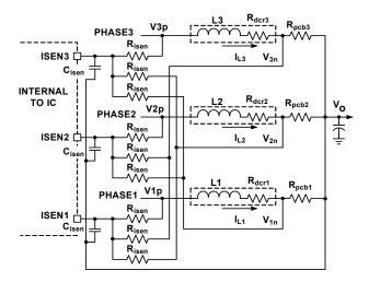
FIGURE 18. DIFFERENTIAL-SENSING CURRENT BALANCING CIRCUIT
