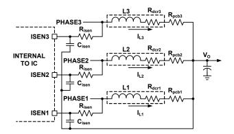
FIGURE 17. CURRENT BALANCING CIRCUIT
