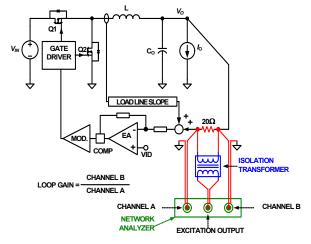
FIGURE 33. LOOP GAIN T2(s) MEASUREMENT SET-UP
