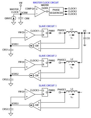
FIGURE 9. R3™ MODULATOR CIRCUIT
