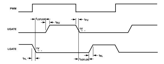
FIGURE 8. GATE DRIVER TIMING DIAGRAM
