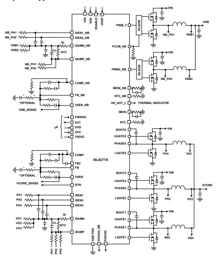
FIGURE 4. TYPICAL APPLICATION CIRCUIT USING INDUCTOR DCR SENSING
