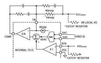
FIGURE 16. DIFFERENTIAL SENSING AND LOAD LINE IMPLEMENTATION
