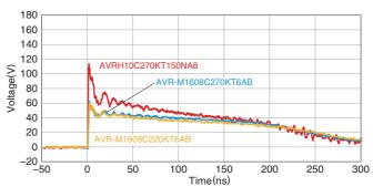
☐Test conditions 150pF/330Ω (IEC61000-4-2) Contact discharge, Charged voltage 8kV
