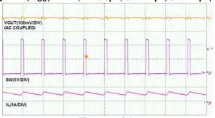
Time- 2µs/div Steady State Test I<sub>OUT</sub> =3A
