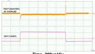
Time- 200μs/div Load Transient Test I<sub>OUT</sub>=1.5A to 3A. Step at 0.8A/μs
