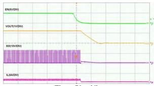
Time- 50µs/div Shutdown Through Enable (I<sub>OUT</sub> =1A)
