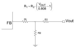
Figure 2. Feedback Divider Network
