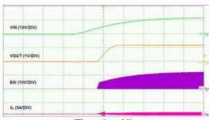
$\label{eq:time-2ms/div} \mbox{Start-up through $V_{\text{IN}}$ (No load)}$
