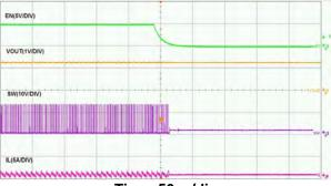
Time- 50µs/div Shutdown Through Enable (No Load)
