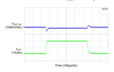
Load Transient (I<sub>OUT</sub>=1A to 2A)
