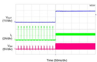
Load Transient (I<sub>OUT</sub>=0.1A to 2A)
