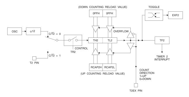
Figure 8-4. Timer 2 in Baud Rate Generator Mode
