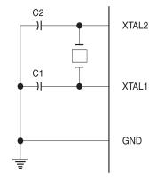
Note: C1, C2 = 30 pF  $\pm$  10 pF for Crystals = 40 pF  $\pm$  10 pF for Ceramic Resonators
