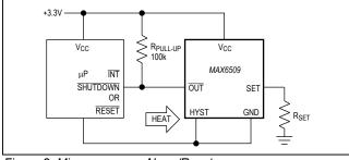
Figure 2. Microprocessor Alarm/Reset
