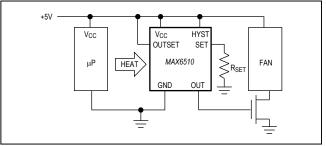
Figure 3. Overtemperature Fan Control
