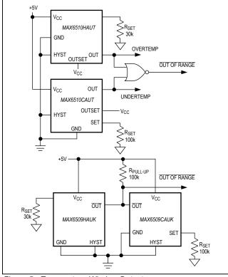
Figure 5. Temperature-Window Detector
