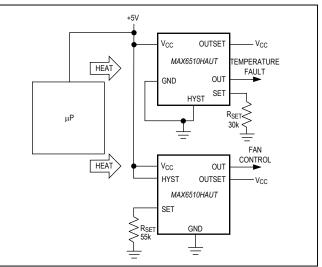
Figure 6. Low-Power, High-Reliability, Fail-Safe Temperature Monitor
